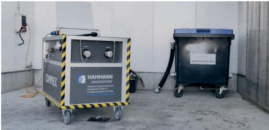
**Fig. 2.** A manufacturer of preforms for PET bottles used an MCU-300-series Compress unit and a corresponding decompression box © Hammann
